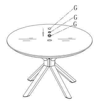
**STEP 3:** Turn the table over and place in desired position. Place parasol bungs & reducers (G) in the hole on table top. You can now use the table.
