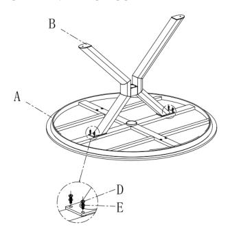
**STEP 1:** Loosely attach left leg frame (B) to table top (A) with big bolts (D) & big flat washers (E), using Allen key (F).
