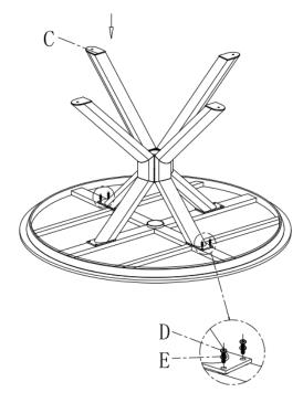
**STEP 2:** Attach right leg frame (C) to table top (A) with big bolts (D) & big flat washers (E), using Allen key (F). Tighten all bolts using Allen key (F) one by one being careful not to over tighten any as this will cause the thread to become damage.
