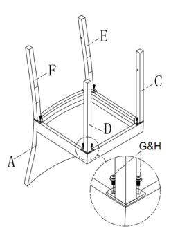
**STEP 1:** Loosely attach front and rear legs (C, D, E and F) to the seating frame (A) with bolts (G) and big flat washers (H) using Allen key (I).
