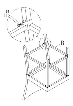
**STEP 2:** Attach connecting rim (B) to the 4 legs with bolts (G) and big flat washers (H) using Allen key (I).
