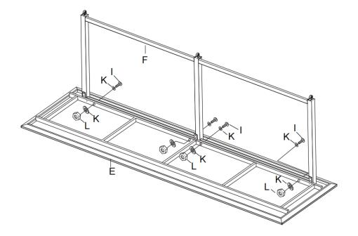
**STEP 4:** Loosely attach dining table leg (F) to dining tabletop (E) with bolts (I), nuts (L) and flat washers (K) using Allen key (N) and spanner (O).
