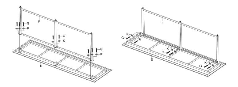
**STEP 3:** Loosely attach dining table leg (F) to dining tabletop (E) with bolts (G) and flat washers (K) using Allen key (N).
