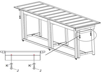
**STEP 5:** Tighten all bolts using Allen key (N) and spanner (O), then turn the assembled dining table over.
