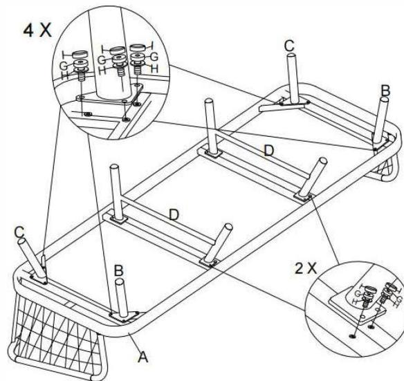
**STEP1:** Attach leg1 (B) ,leg2 (C), Center leg (D) to the Frame (A), using the Bolt M6X20 (G) and Washer (H). Tighten the bolts and cover with the Plastic bolt cap (I).
