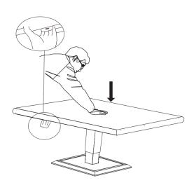
**STEP 6:** Gently press down on the centre of the table while squeezing the handle to lower the table.
