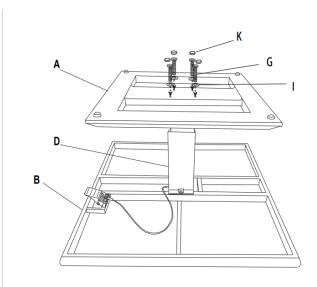
**STEP 3:** Attach bottom (A) to the gas pump (D), using the M8x50 bolt (G) and washer (I). Tighten all the bolts with the Allen key (M), and cover with the plastic bolt cap (K).
