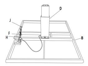
**STEP 1:** Attach gas pump (D) to the table top (B), using the M6x25 bolt (E) and washer (H). Tighten all the bolts with the Allen key(L), and cover with the plastic bolt cap (J).
