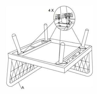
**STEP1:** Attach Leg2 (C) to the Frame (A), using the Bolt M6X20 (G) and Washer (H). Tighten the bolts and cover with the Plastic bolt cap (I)
