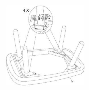
**STEP1:** Attach Leg1 (B) to the Frame (M), using the Bolt M6X20 (G) and Washer (H). Tighten the bolts and cover with the Plastic bolt cap (I)
