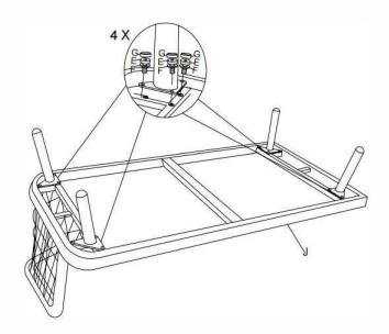
**STEP1:** Attach Leg (B) to the Frame (J), using the Bolt M6X20 (E) and Washer (F). Tighten the bolts and cover with the Plastic bolt cap (G)
