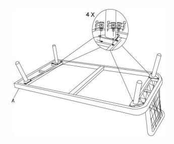
**STEP1:** Attach Leg (B) to the Frame (A), using the Bolt M6X20 (E) and Washer (F). Tighten the bolts and cover with the Plastic bolt cap (G)
