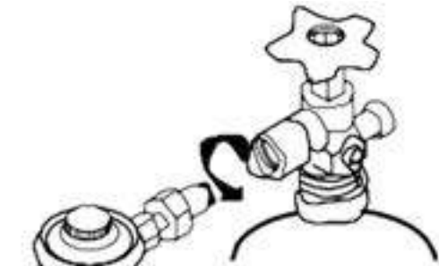
For POL cylinders, tighten anti-clockwise
