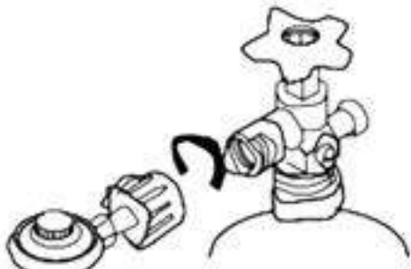
For Quick Connect cylinders, tighten clockwise
